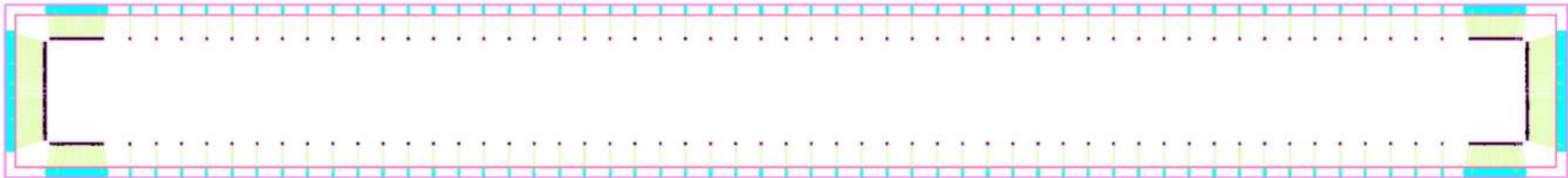
Fig: Die in the cavity with tentative bond pad layout
